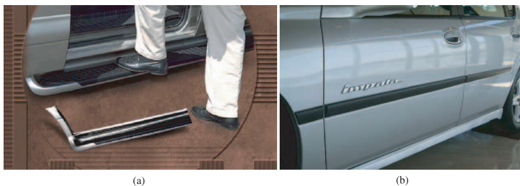
Figure 9. TPO nanocomposites: application for automotive parts [109]: (a) M-Van step Assist: 1st commercial launch and (b) Impala: 2nd nanocomposite application. Through the courtesy of M. Verbrugge, General Motors.
