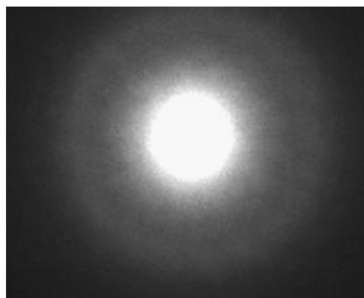
Fig. 6. The selected area diffraction pattern of the Ni-P coating on Mg-10Gd-4.8Y-0.6Zr alloy.
