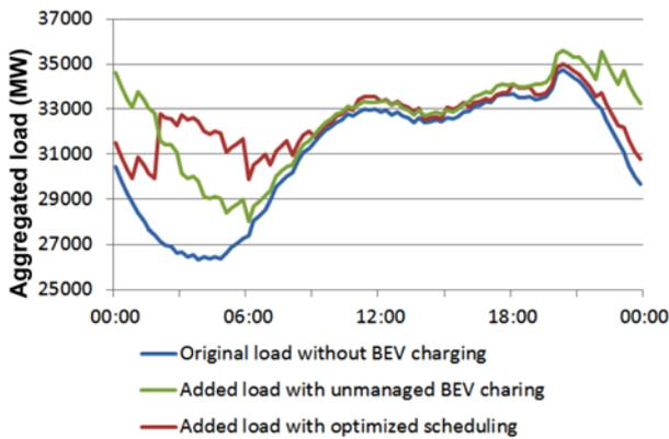
Figure 8. Comparison of added load distribution between unmanaged BEVs versus managed BEVs.
