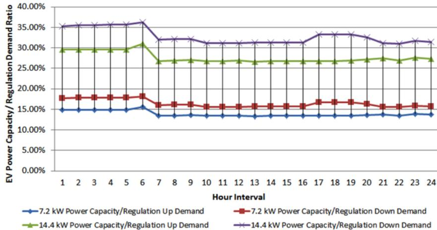
Figure 7. Hourly trend of the ratio of EV power capacity/total regulation demand.
