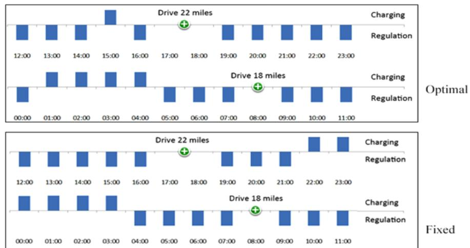
Figure 3. Comparison of optimized and fixed charge/discharge schedule in the next 24 hours.
