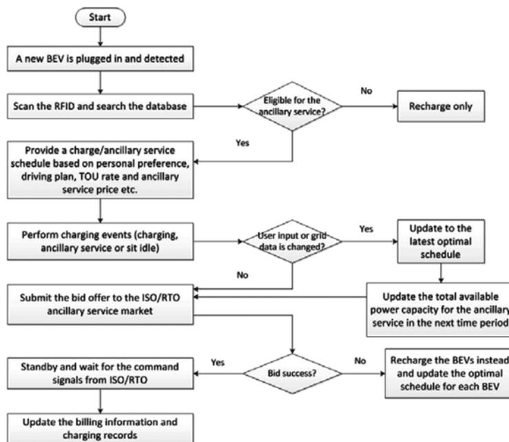
Figure 2. Event sequence diagram of the smart charge scheduling model.
