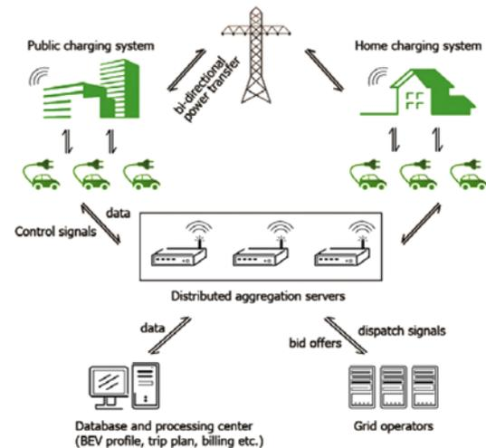
Figure 1. Components and communication architecture in the smart charging system.
