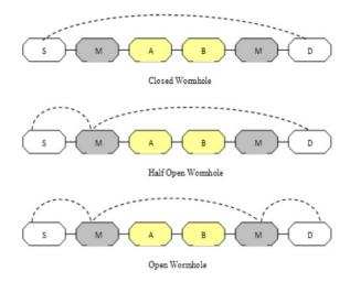
Figure 1 worm hole attack and types
