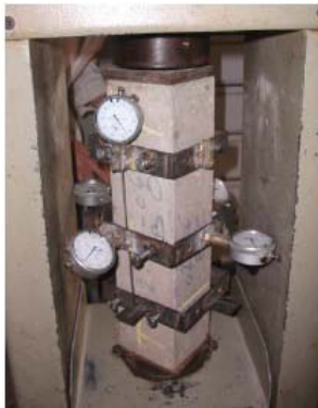
Figure 2: The site of the executives and indicators on the test-tube
