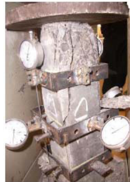
Figure 3: Deformations measured on the test-tube during compression
