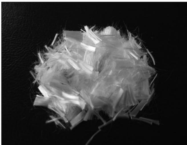
Fig. 3. Polypropylene fibers applied in this research.
