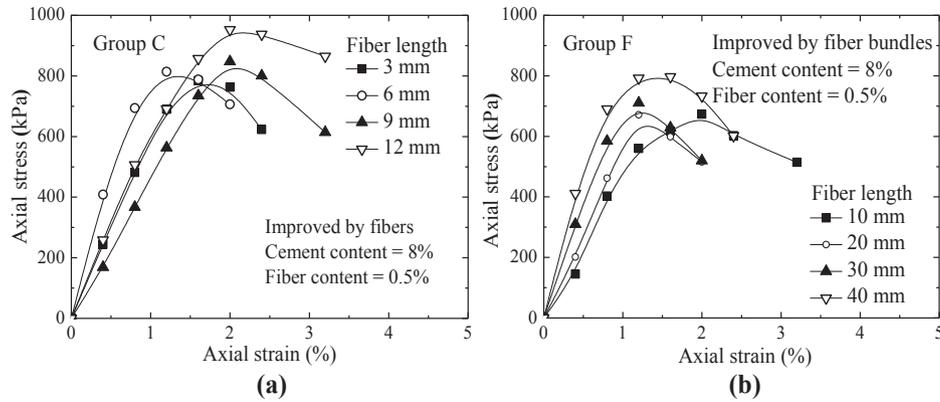
Fig. 8. Stress–strain curves for specimens improved with different fiber lengths under cement content 8% and fiber content 0.5%: a) fibers and b) fiber bundles.
