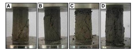
Fig. 11. Effects of silica fume, fiber and silica fume–fiber mixtures on the failure characteristics; (A) natural clayey soil, (B) 20% silica fume–modified clayey soil, (C) 2% fiber-modified clayey soil and (D) 20% silica fume and 2% fiber-modified clayey soil.
