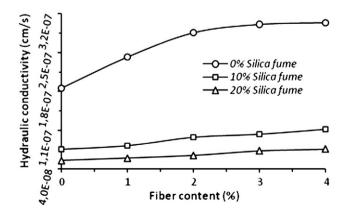
Fig. 12. Effect of the silica fume and fiber on the hydraulic conductivity.
