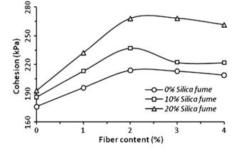
Fig. 9. Effect of the scrap tire rubber fiber on the cohesion.
