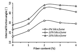
Fig. 10. Effect of the scrap tire rubber fiber on the internal friction angle.
