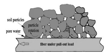
**Fig. 7.** Sketch drawing of interfacial mechanical interactions between soil particles and fiber (modified from Tang et al., 2010).
