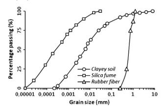
Fig. 1. The grain-size distributions of clayey soil, silica fume and scrap tire rubber fiber.
