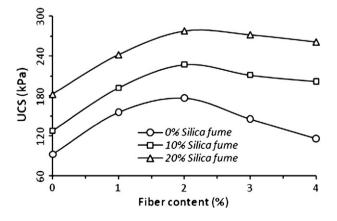
Fig. 5. Effect of the scrap tire rubber fiber on the UCS.
