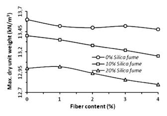
Fig. 3. Effect of the scrap tire rubber fiber on the maximum dry unit weight.
