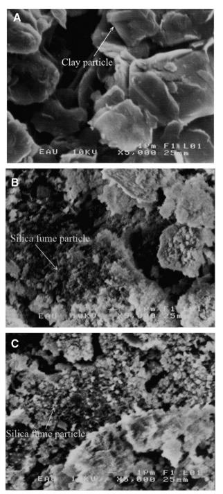
Fig. 14. Images of silica fume-modified clayey soil with (A) 0% silica fume, (B) 10% silica fume and (C) 20% silica fume.
