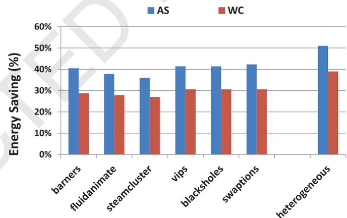
Fig. 10. Energy saving obtained for ms-WiNoC with 64 nodes under different traffic scenarios and for the heterogeneous platform of the case study.
