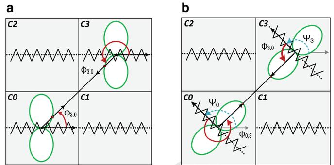
**Fig. 2.** Reciprocal antennas orientation and directivity functions. The directivity between C0 and C3 improves from configuration (a) to configuration (b).
