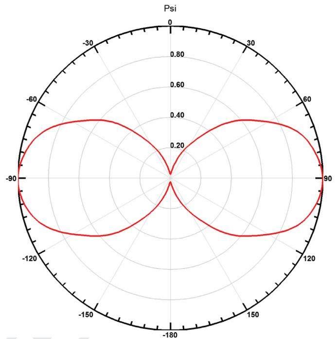
**Fig. 4.** Radiation pattern for a zigzag antenna at the elevation of maximum radiation ( $\phi = 100^\circ$ ).  $\theta = 0^\circ$  is the direction orthogonal to the antenna's main axis. According to Fig. 1, we assume the antenna situated upon the XY plane (coplanar with silicon die).
