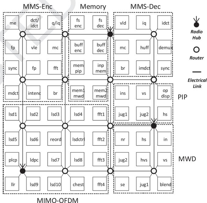
Fig. 8. Heterogeneous system composed by a multimedia sub-system, a MIMO-OFDM receiver, a PIP and a MWD module.
