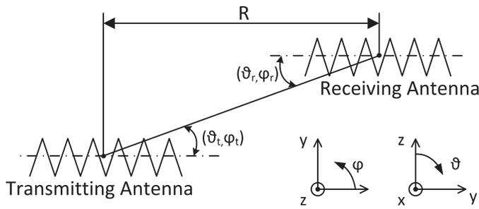
**Fig. 1.** Friis transmission equation: geometrical orientation of transmitting and receiving antennas. As indicated, considering a spherical coordinate system,  $\phi$  is the azimuthal angle in the XY plane, where the X-axis is  $0^\circ$  and Y-axis is  $90^\circ$ .  $\theta$  is the elevation angle where the Z-axis is  $0^\circ$ , and the XY plane is  $90^\circ$ .
