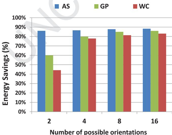
Fig. 7. Energy saving for various number of possible orientations of the antenna (WiNoC configured with 16 radio hubs).
