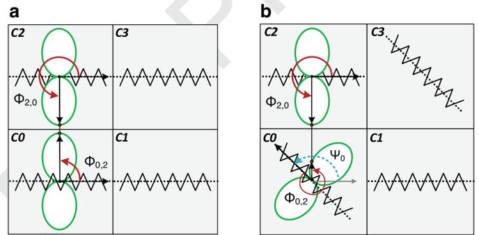
**Fig. 3.** Reciprocal antennas orientation and directivity functions. Configuration (a) improves communication energy between tiles C0 and C2 whereas configuration (b) improves communication energy between tiles C0 and C3.
