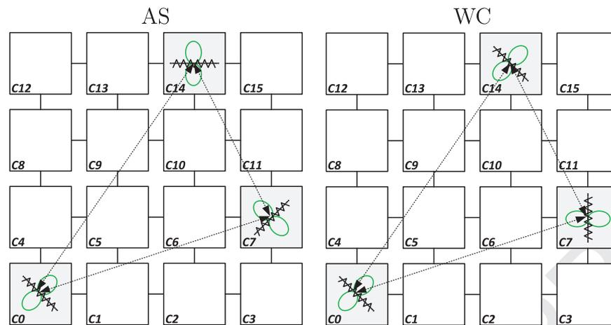
Fig. 9. Optimal antennas orientations found by the simulated annealing algorithm for the application specific (AS) and worst case (WC) scenarios.
