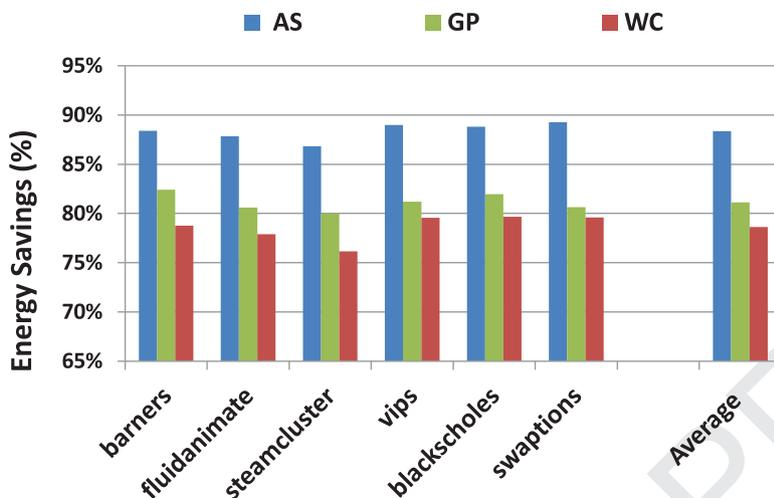
Fig. 5. Energy saving obtained for ms-WiNoC with 256 nodes under different traffic scenarios.
