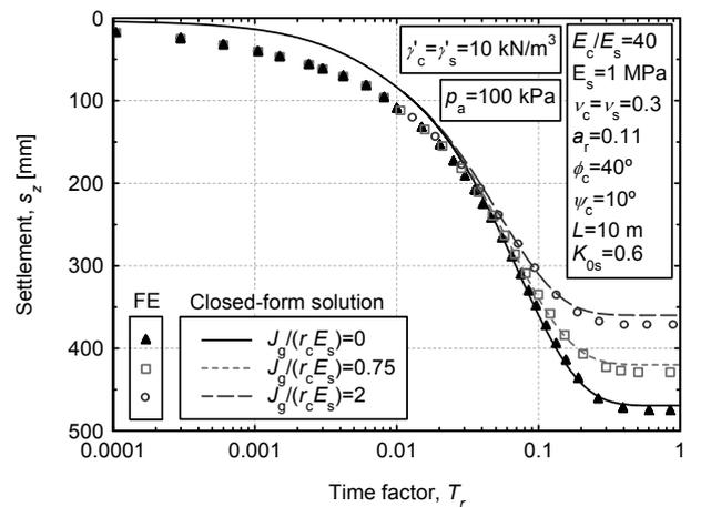
Figure 6. Time-settlement curve.
