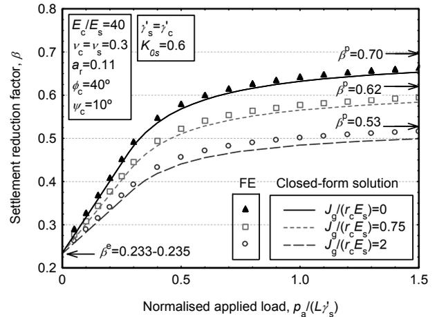
Figure 4. Settlement reduction. Influence of the applied load.
