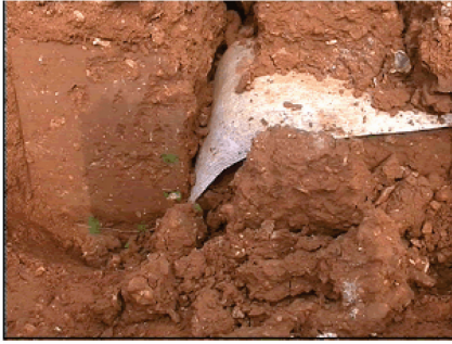
Figure 8. Failure of rectangular trench in flint clay.
