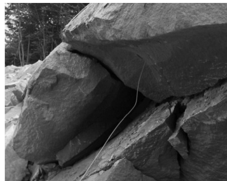
Fig. 5. Intact stemming zones indicating face burst flyrock mechanism.
