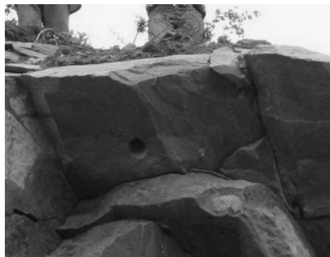
Fig. 5. Intact stemming zones indicating face burst flyrock mechanism.
