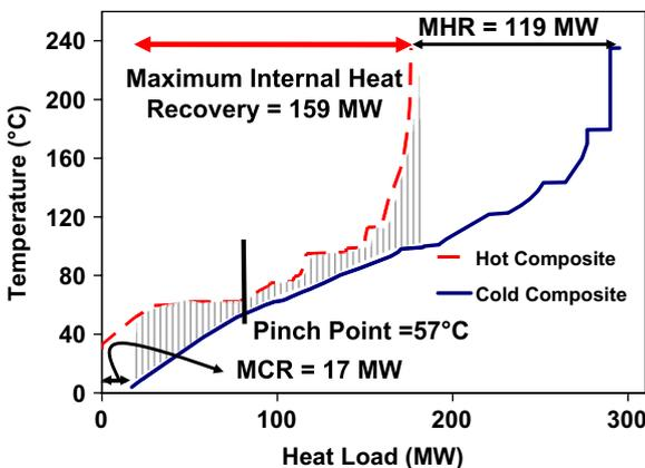
Fig. 5. Thermal composite curves of the process after water reutilization.
