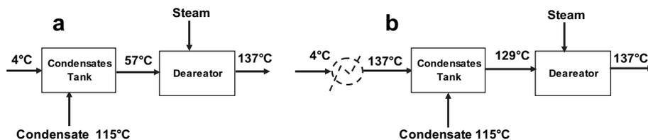
**Fig. 10.** a) Current deaeration system; b) retrofit system.
