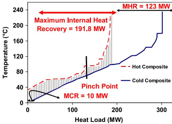
Fig. 4. Thermal composite curves of the process in initial configuration.
