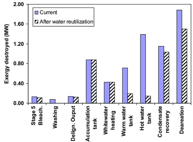
**Fig. 9.** Exergy destroyed for different NIM points: current and after water reutilization configuration.
