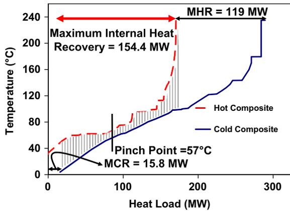
Fig. 11. Thermal composite taking into account the elimination of NIM points (HEN-3).
