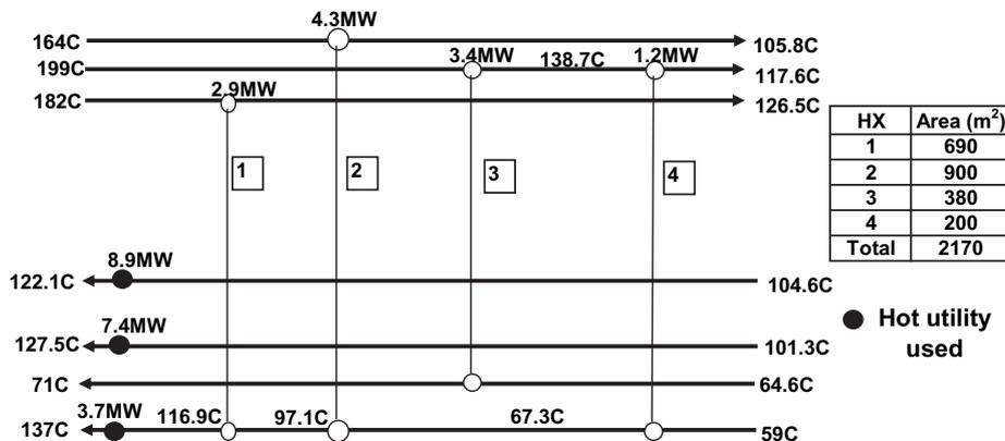
Fig. 12. HEN-3: network design above the pinch [36].
