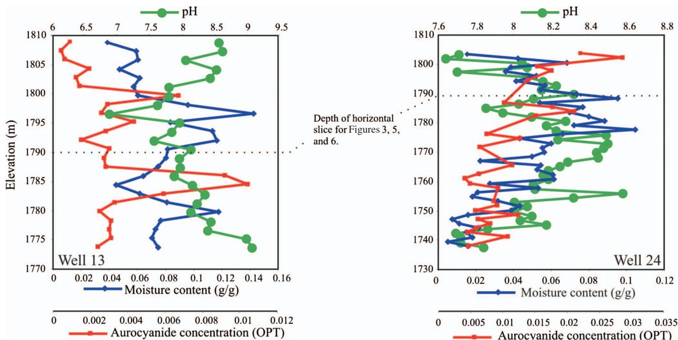
Figure 2. Example data distribution of moisture, leachable gold (as aurocyanide), and pH within two wells, 13 and 24. A moisture content of 0.005 is dry, whereas 0.28 is moist ore.
