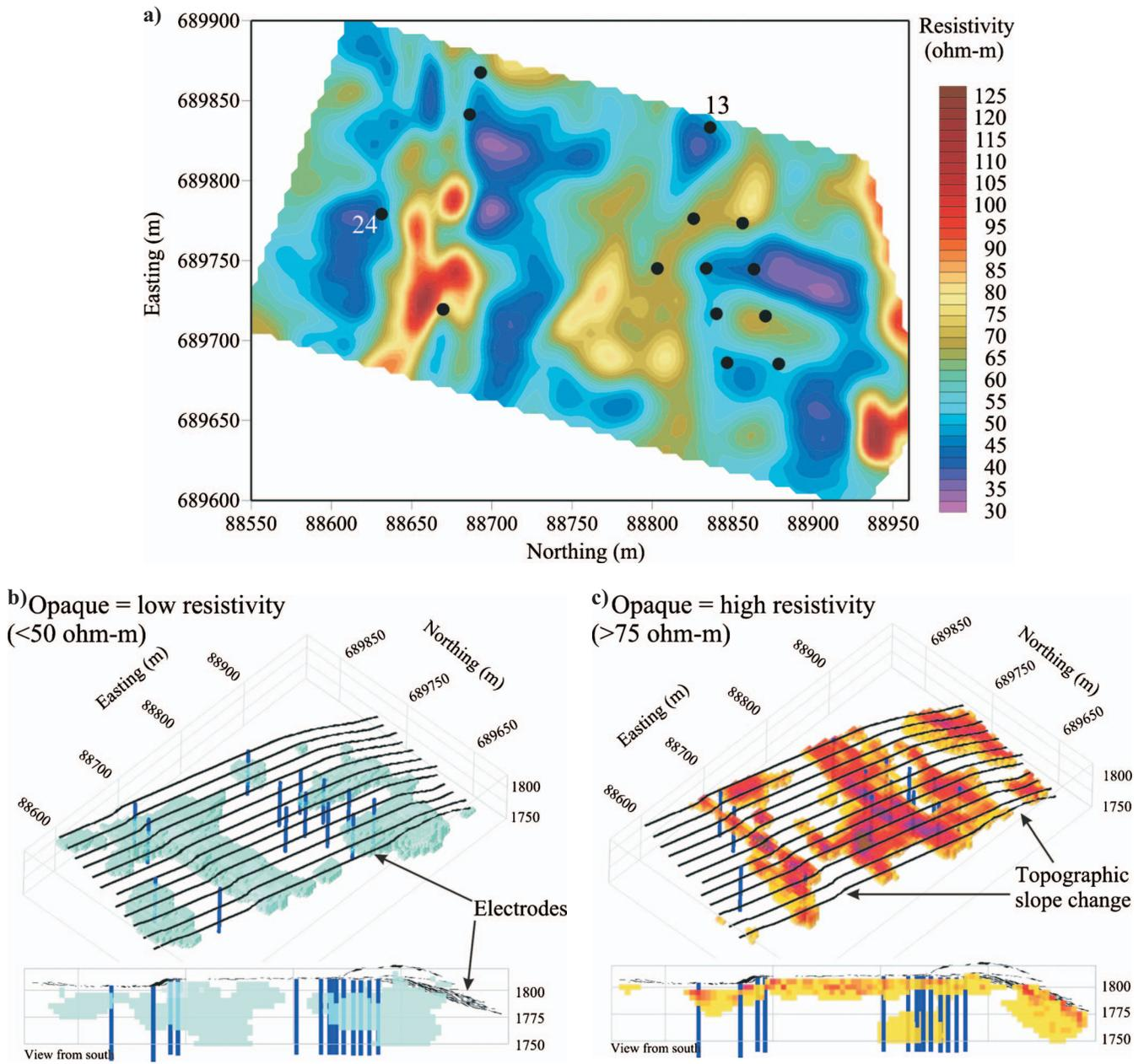
Figure 4. Electrical resistivity distribution within the NAL pad, showing (a) a horizontal slice at an elevation of 1790 m and solid model renderings of (b) low resistivity and (c) high resistivity material. Black lines draped across the surface in (b) and (c) represent electrode locations and give an indication of topography. Coordinates are in Nevada State Plane, meters, North American datum of 1927.
