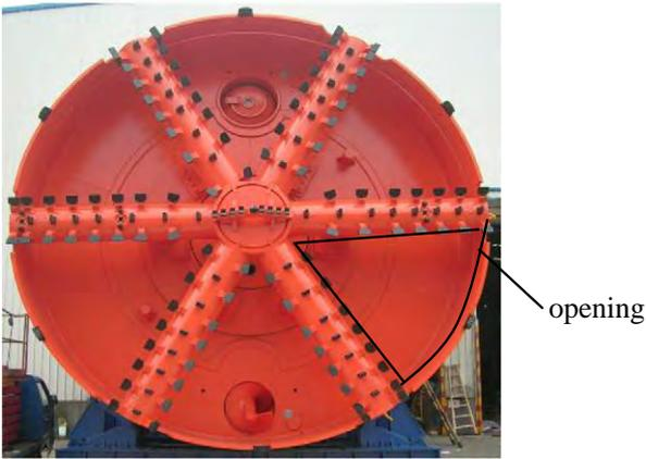
Fig. 3. Cutterhead of different opening ratios.
