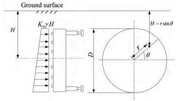
Fig. 5. Diagram of forces acting on the cutterhead.
