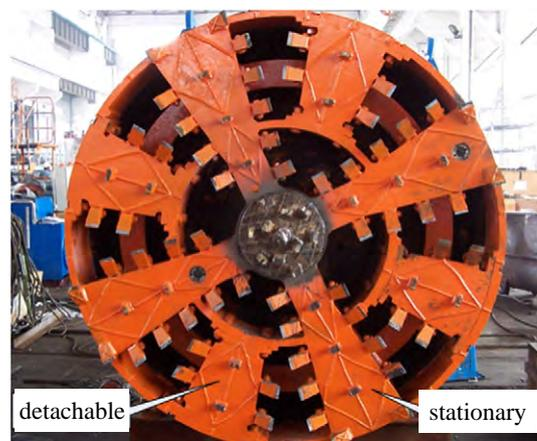
Fig. 9. Cutterhead used in experiment.
