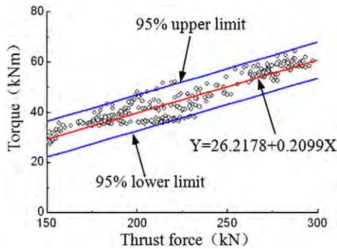
Fig. 14. Relation between torque and thrust force.
