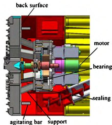
Fig. 4. Structure of cutterhead of EPB shield.
