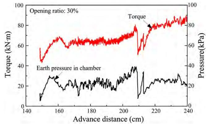
Fig. 12. Relation between torque and earth pressure in chamber.
