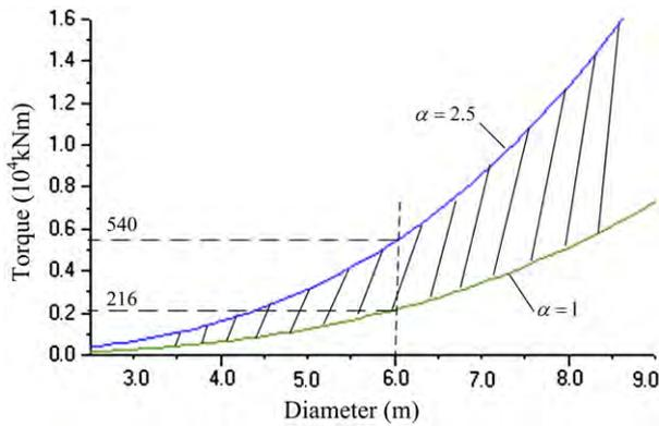
Fig. 1. Torque/diameter characteristics of EPB shield.
