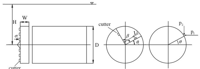
Fig. 7. Diagram of forces acting on cutters.
