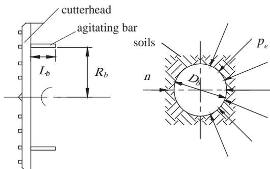
Fig. 8. Diagram of force acting on the agitating bar.
