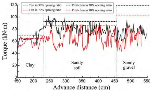
Fig. 11. Torque variations with different opening ratios.
