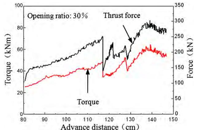
Fig. 13. Variations of torque and thrust force in clay.
