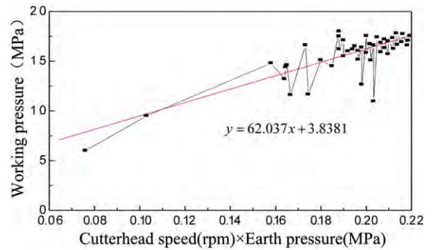
Fig. 2. Relation between torque and product of speed and earth pressure.
