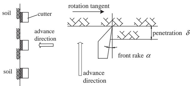
Fig. 6. Schematic of cutting process.
