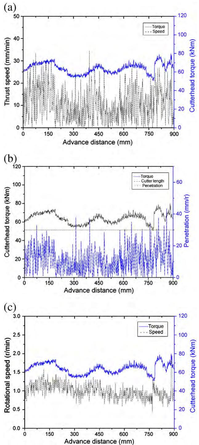
Fig. 15. Effects of thrust and cutting on cutterhead torque.
