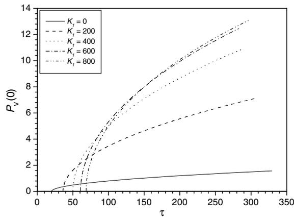
Fig. 5.  $P_1(0)$  versus temperature rise  $\tau$  for different values of  $K_1$  ( $K_2 = 0$ , mode 1).
