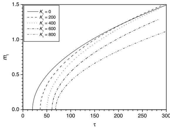
Fig. 4. End bending moment  $m_1$  versus temperature rise  $\tau$  for some values of  $K_1$  ( $K_2 = 0$ , mode 1).
