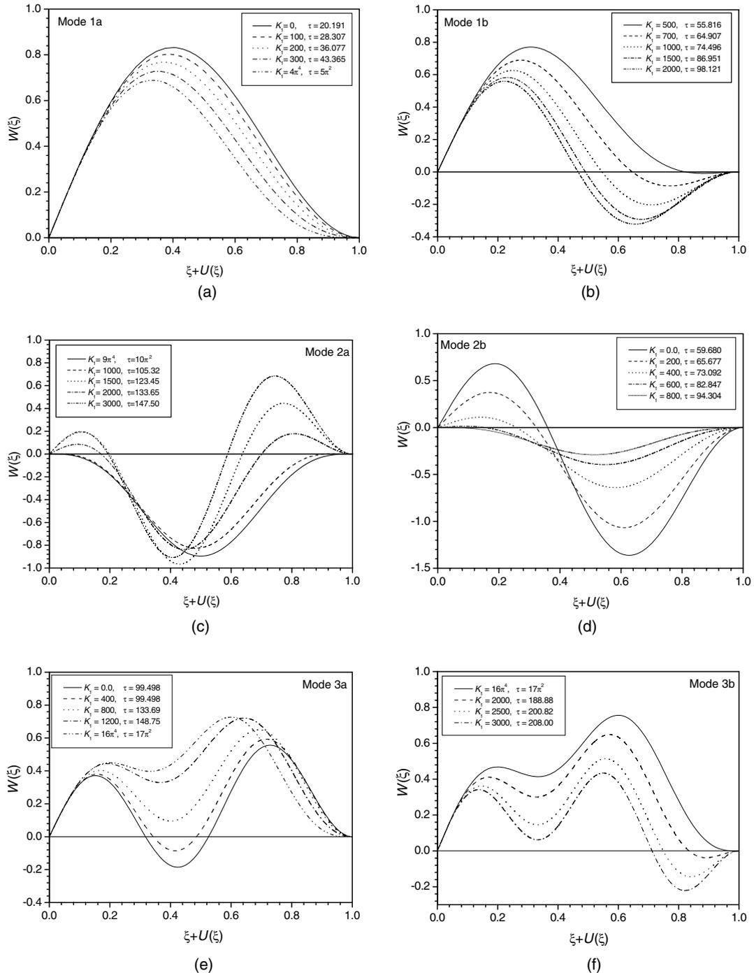
Fig. 2. Critical buckling mode shapes of the pinned–fixed beam for some specified values of  $K_1$ . (a) Mode 1a, (b) mode 1b, (c) mode 2a, (d) mode 2b, (e) mode 3a, and (f) mode 3b.
