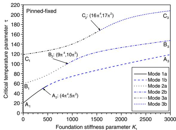
Fig. 1. Characteristic curves of the critical buckling temperature  $\tau$ , versus foundation stiffness parameter  $K_1$ , for the first three buckling modes.
