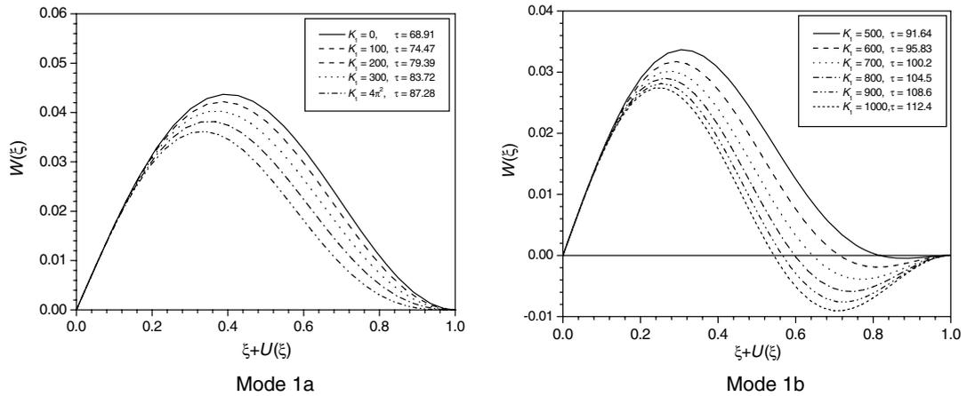
Fig. 6. Thermal post-buckling configurations of the beam in the first mode for different values of  $K_1$  and  $\tau$  ( $K_2 = 0, \beta = 10^\circ$ ).
