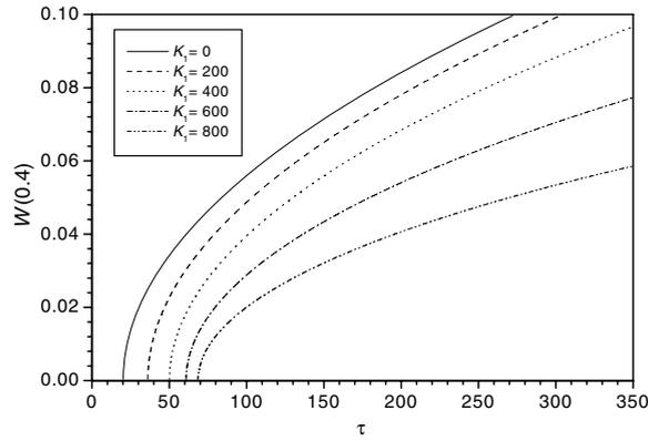
Fig. 3. Dimensionless deflection,  $W(0.4)$ , versus temperature rise  $\tau$  for some specified values of  $K_1$  ( $K_2 = 0$ , mode 1).
