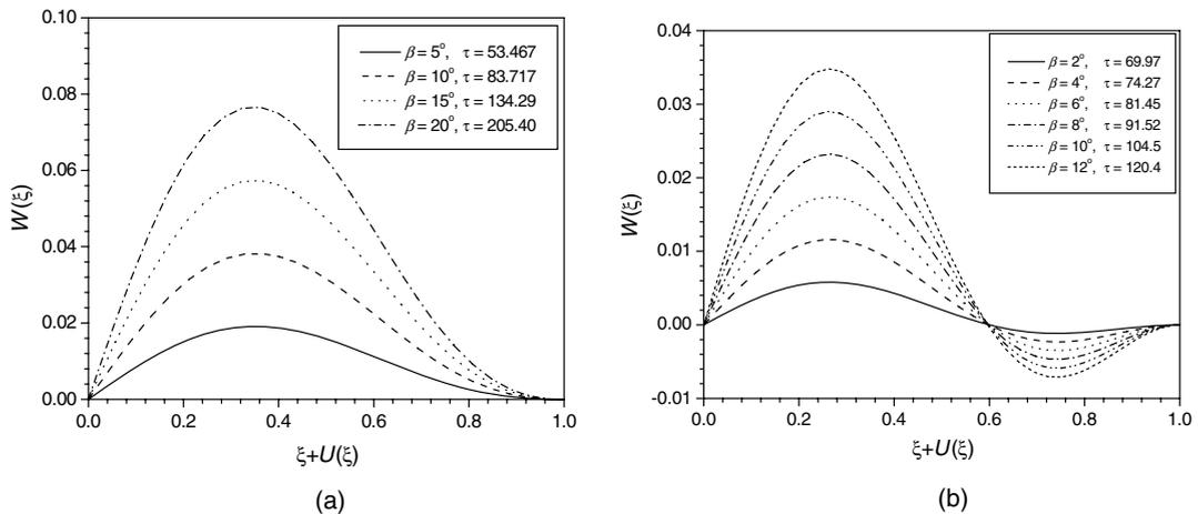
Fig. 7. Thermal post-buckling configurations of the beam in the first mode for different values of  $\beta$  and  $\tau$ . (a)  $K_1 = 300, K_2 = 0$  and (b)  $K_1 = 800, K_2 = 0$ .
