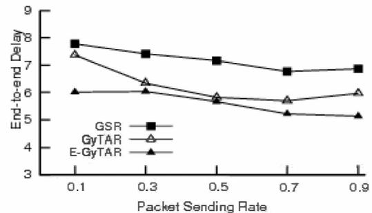
Figure 5. End-to-end delay vs. packet sending rate (175 nodes)
