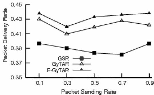
Figure 3. Delivery ratio vs. packet sending rate (175 Nodes)
