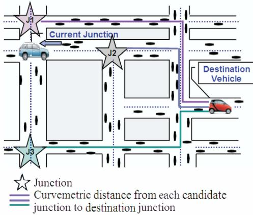
Figure 1. Problem in GyTAR junction selection mechanism.
