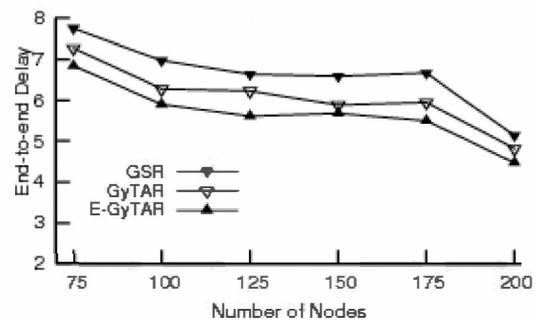
Figure 6. End-to-end delay vs. number of nodes at 5 packets/sec
