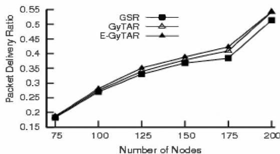
Figure 4. Delivery ratio vs. number of nodes at 5 packets/sec
