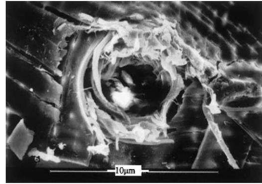
Fig. 6. Hole used as transport channel and fibers remained continuous.
