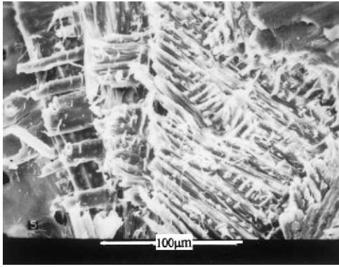
Fig. 4. The dual helicoidal arrangement of plies.
