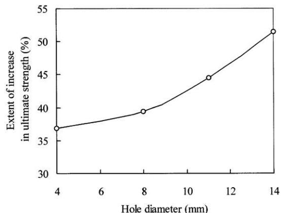
Fig. 9. Extent of the increase in the ultimate strength of the specimens with preformed holes of different hole-diameters.
