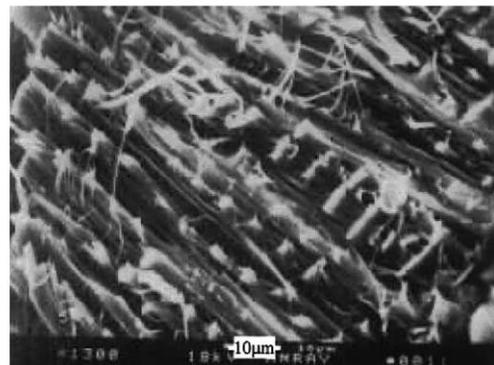
Fig. 7. Spaces and pillars between plies of fiber.
