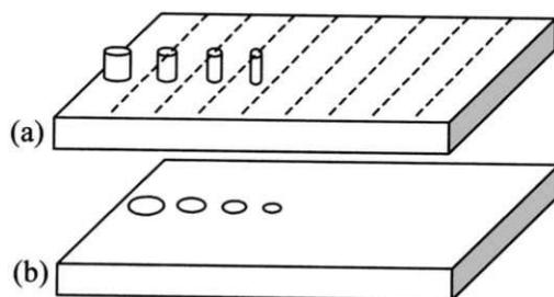
Fig. 8. (a) The bottom mould board containing different diameter circular pins, (b) The upper mould board with matched holes.
