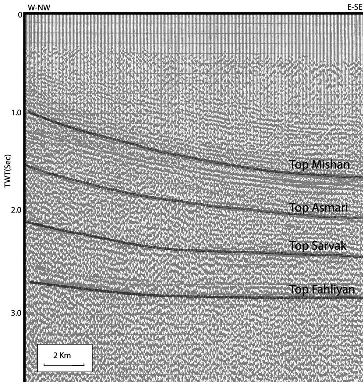
Fig. 7. Interpreted seismic reflection profile through the northern flank of Binak anticline, showing thickness variations at the crest of the anticline in the Neocomian–Lower Miocene time interval. For location, see Fig. 6, II. It might be related to the influence of deep seated NS fault (Kharg–Mish) on sedimentation by causing flexure in sedimentary basin.
