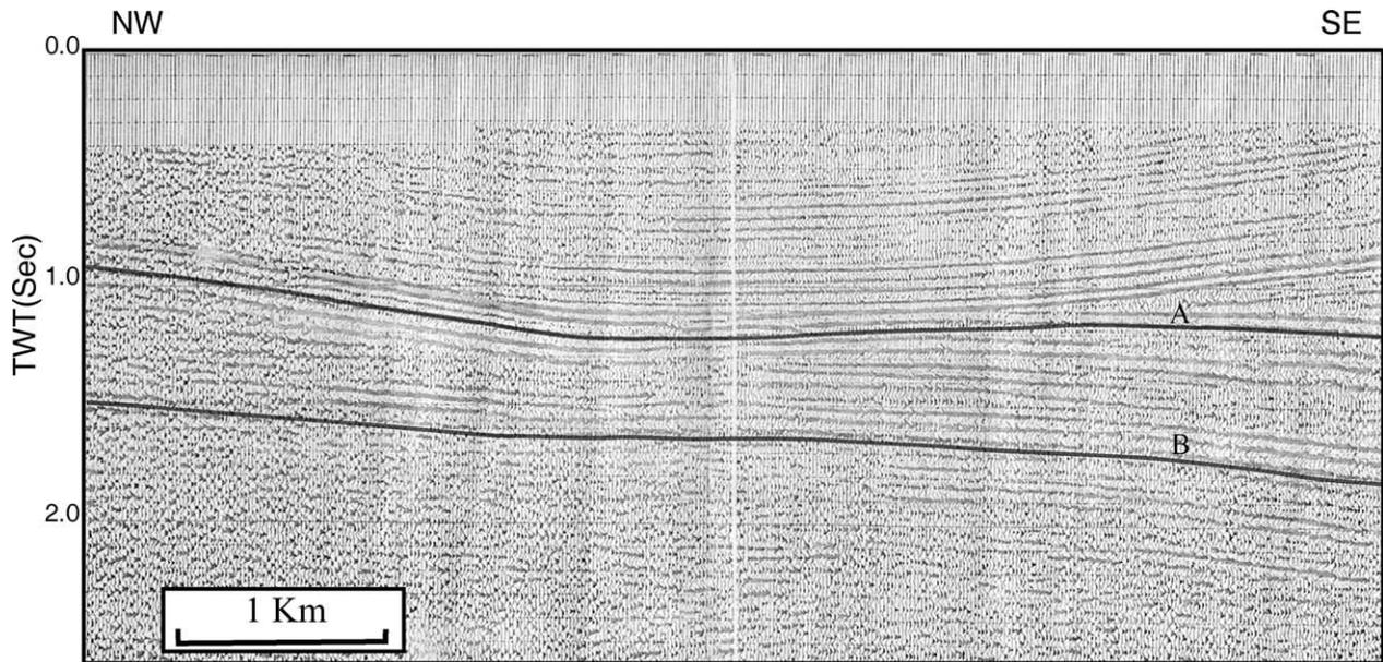
Fig. 11. Interpreted seismic profile through the Hendijan–Bahregansar fault between the Aghajari and Pazanan anticlines. It shows clear thickness changes during the Middle Cretaceous–Lower Miocene time interval. For location, see Fig. 6, III. Both of anticlines were drilled down to the Lower Cretaceous, and no fault or disharmonic features were reported. (A) Top Asmati Fm., (B) Top Fahliyan Fm.
