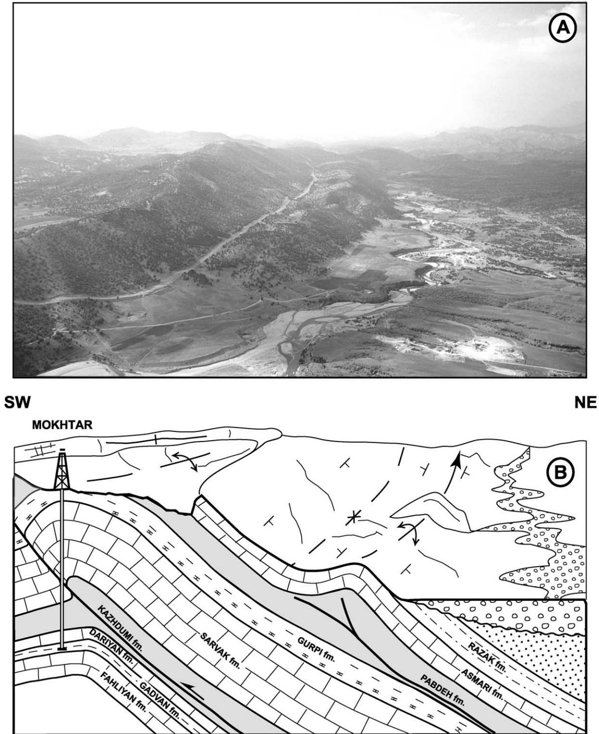
Fig. 4. (A) Photograph of Mokhtar anticline, (B) Line drawing and section of the Mokhtar anticline. The Mokhtar well proved thickening and thrusting of the Albian shales (Kazhdumi fm.) in the core of the structure. ‘Rabbit ear’ structures on the flank of the main fold show the influence of intermediate décollement level (Eocene Pabdeh Fm.) on fold style.
