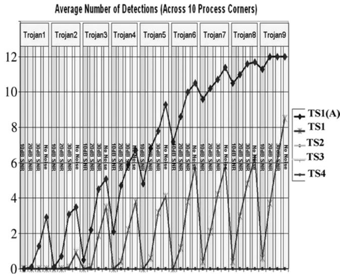
Fig. 7. Number of detections for TS1\_Active, TS1\_Passive (the original passive stimulus), and the variants TS2, TS3, and TS4 that add random undesired switching activity to the circuit.
