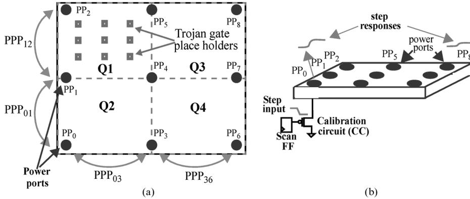
Fig. 1. (a) Architecture of the simulation model, each of the quads (Q1–Q4) contains a copy of C499 benchmark; (b) calibration circuit (CC) and step.
