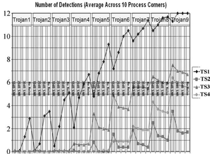
Fig. 6. Number of detections for TS1, the original active stimulus, and for the three variants TS2, TS3, and TS4 that add random background switching activity to the circuit.
