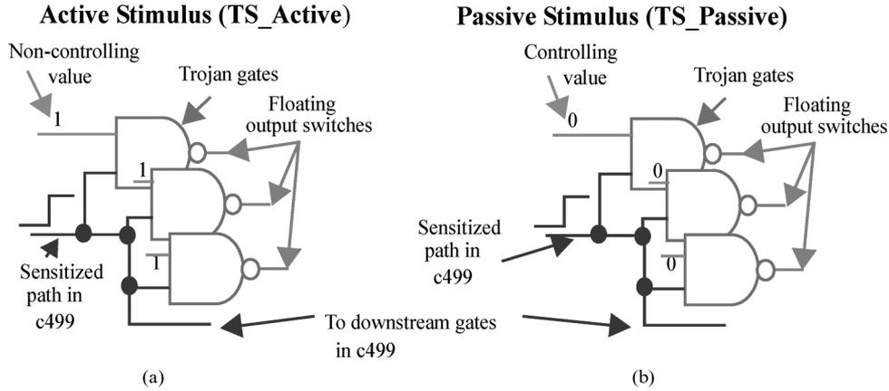
Fig. 3. Trojan gate sensitization criteria under the two test sequences [4].
