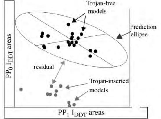
Fig. 2. Example scatterplot for power port pairing PP0 and PP1 (referred to as PPP01) [5].
