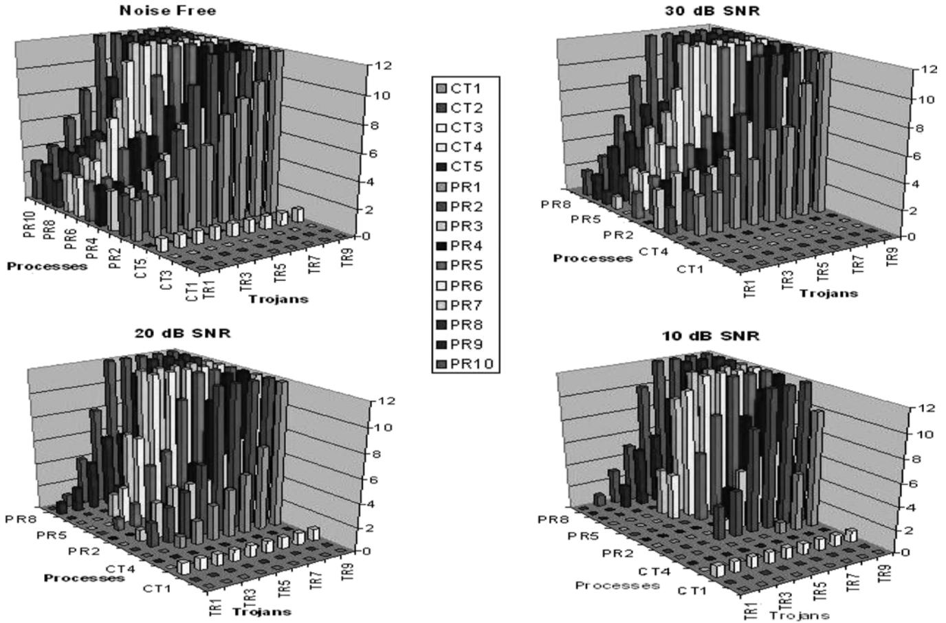
Fig. 4. Number of detections under TS\_Active stimulus for noise-free and three different noise levels.
