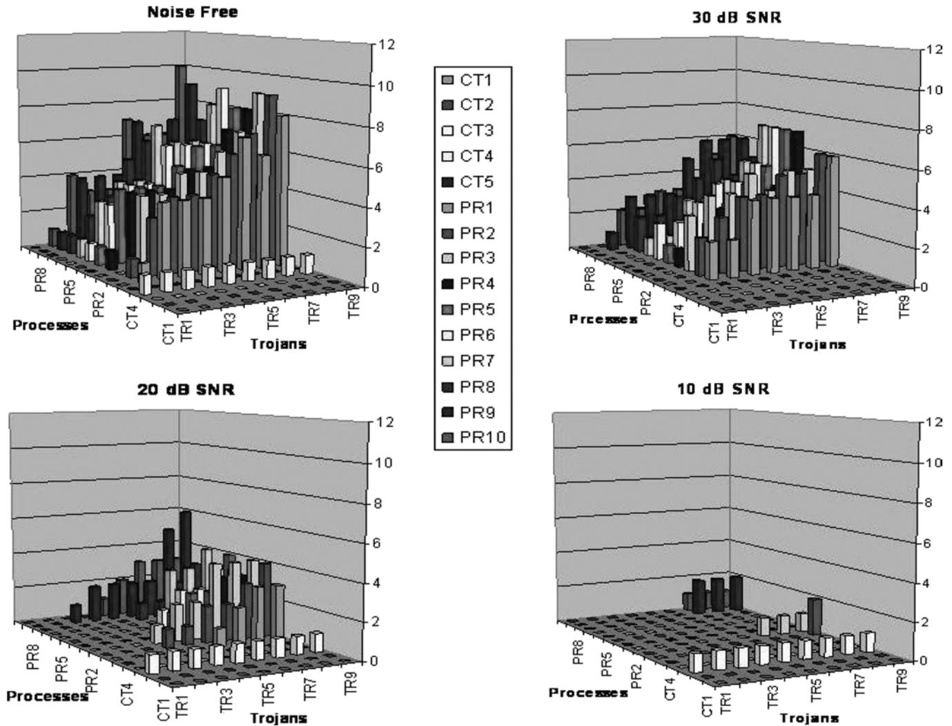
Fig. 5. Number of detections under TS<sub>Passive</sub> stimulus for noise-free and three different noise levels.
