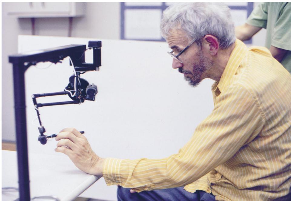
Fig. 1. Dr. Stanley Swanson juxtaposed with the PHANToM manipulator. Small positional sensors and servomotors are barely visible. This photograph makes it possible to visualize the translational latitude (ca. 20 cm) available for interactive input/output.
