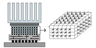
Fig. 2. 3D grid of a chip for thermal modeling
