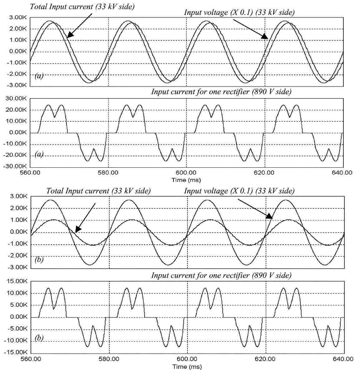
Fig. 4. Diode rectifiers input waveforms. (a)  $P = 100$  MW. (b)  $P = 40$  MW.
