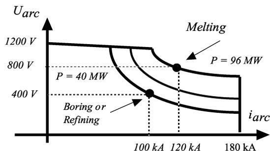
Fig. 6. Output characteristic of the chopper dc supply during the tap-to-tap time.
