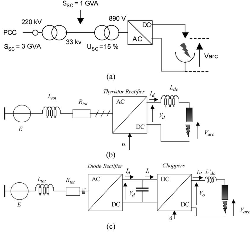
Fig. 9. (a) Structure of power supply for a dc arc furnace. (b) Equivalent circuit for one thyristor rectifier. (c) Equivalent circuit for one diode rectifier associated with choppers.
