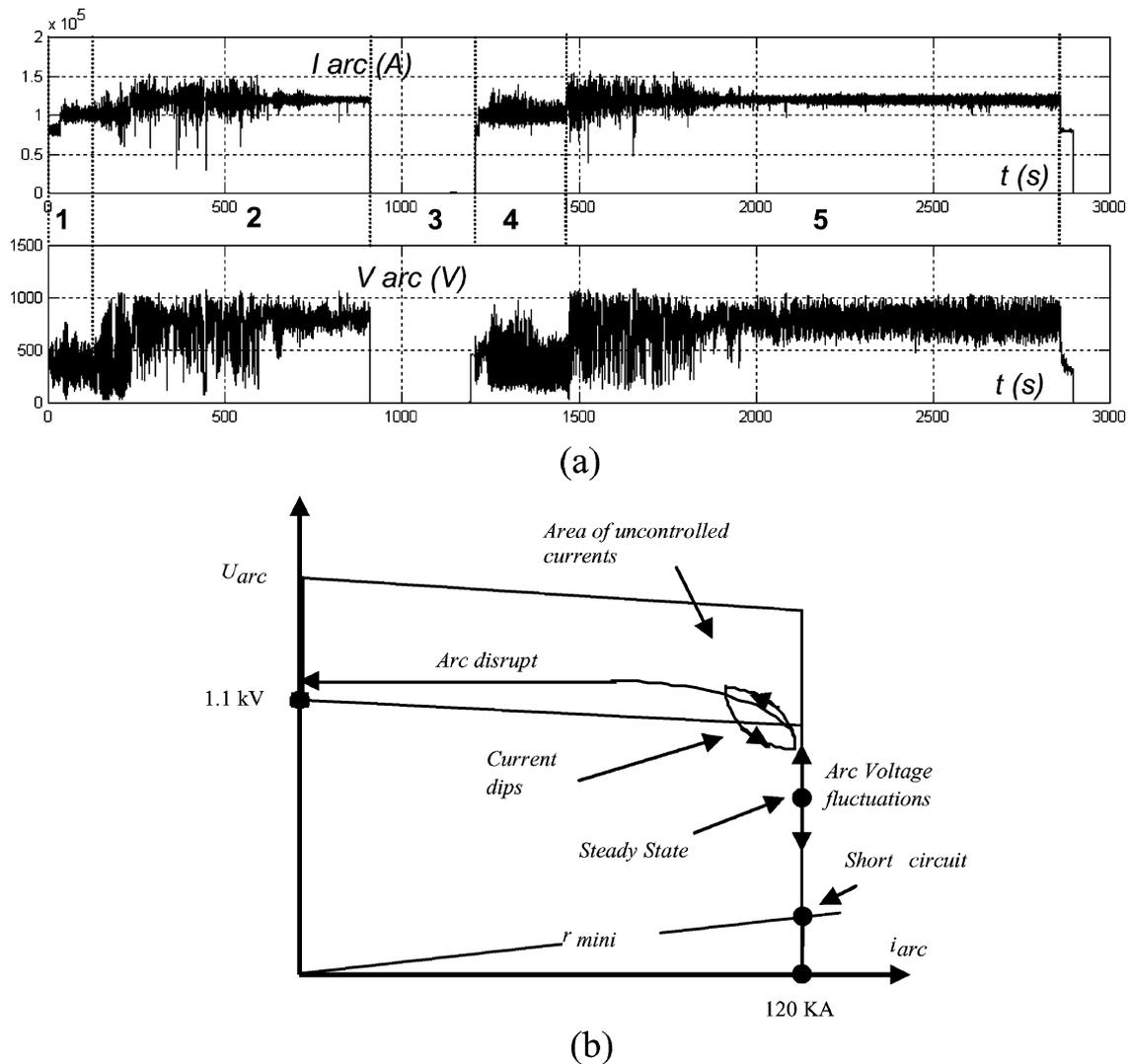
Fig. 2. (a) Current and voltage waveforms for a classical dc arc furnace. (b) Output characteristic of a classical supply.
