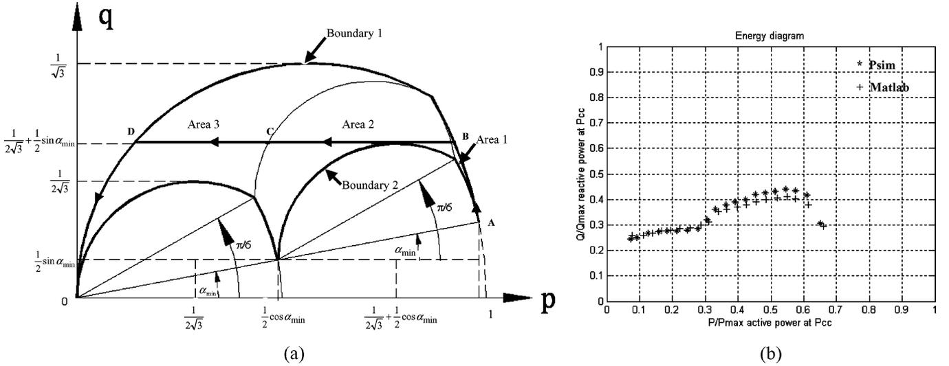
Fig. 3. Thyristor rectifier with neutral-point freewheel diodes. (a)  $q = f(p)$  theoretical diagram. (b) Simulation results  $q = f(p)$  diagram at PCC.
