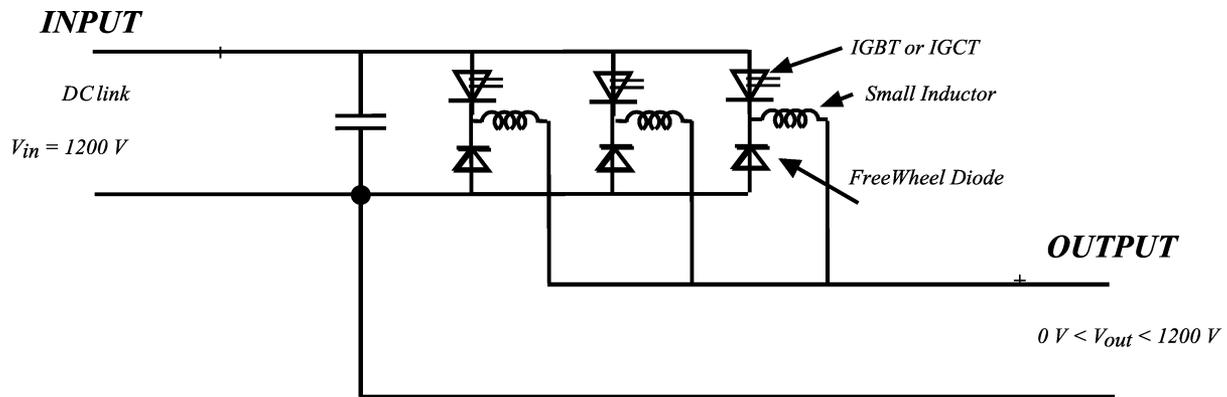
Fig. 7. Buck converters in parallel association.
