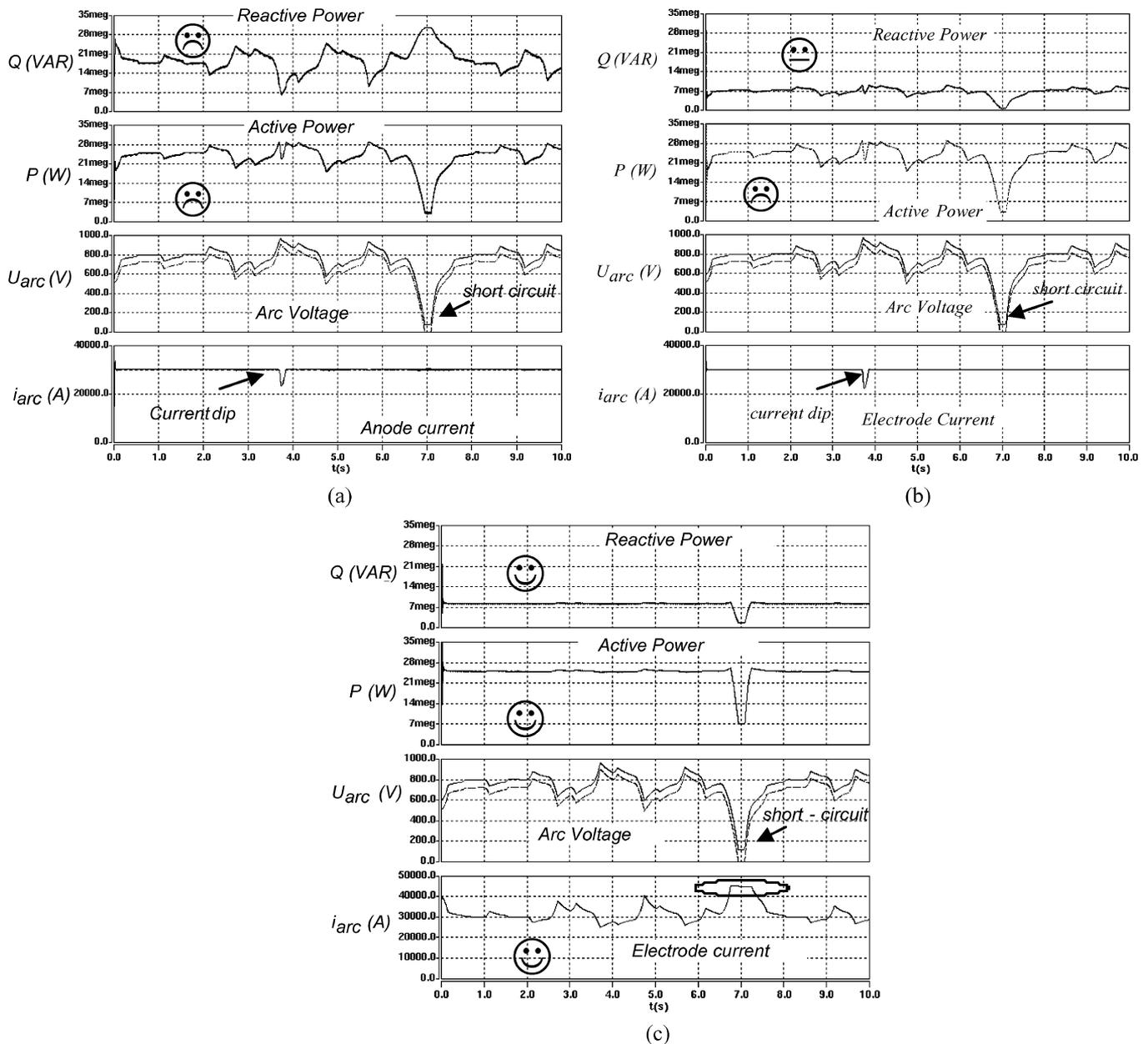
Fig. 5. Simulation waveforms for one anode. (a) Classical supply with thyristor rectifiers. (b) Chopper solution with constant current control. (c) Chopper solution with constant power control.
