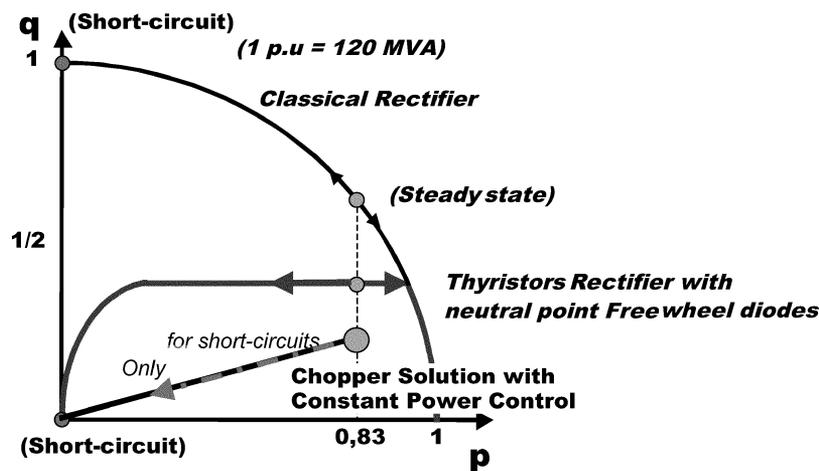
Fig. 8. Reactive power versus active power ( $q = f(p)$ ).
