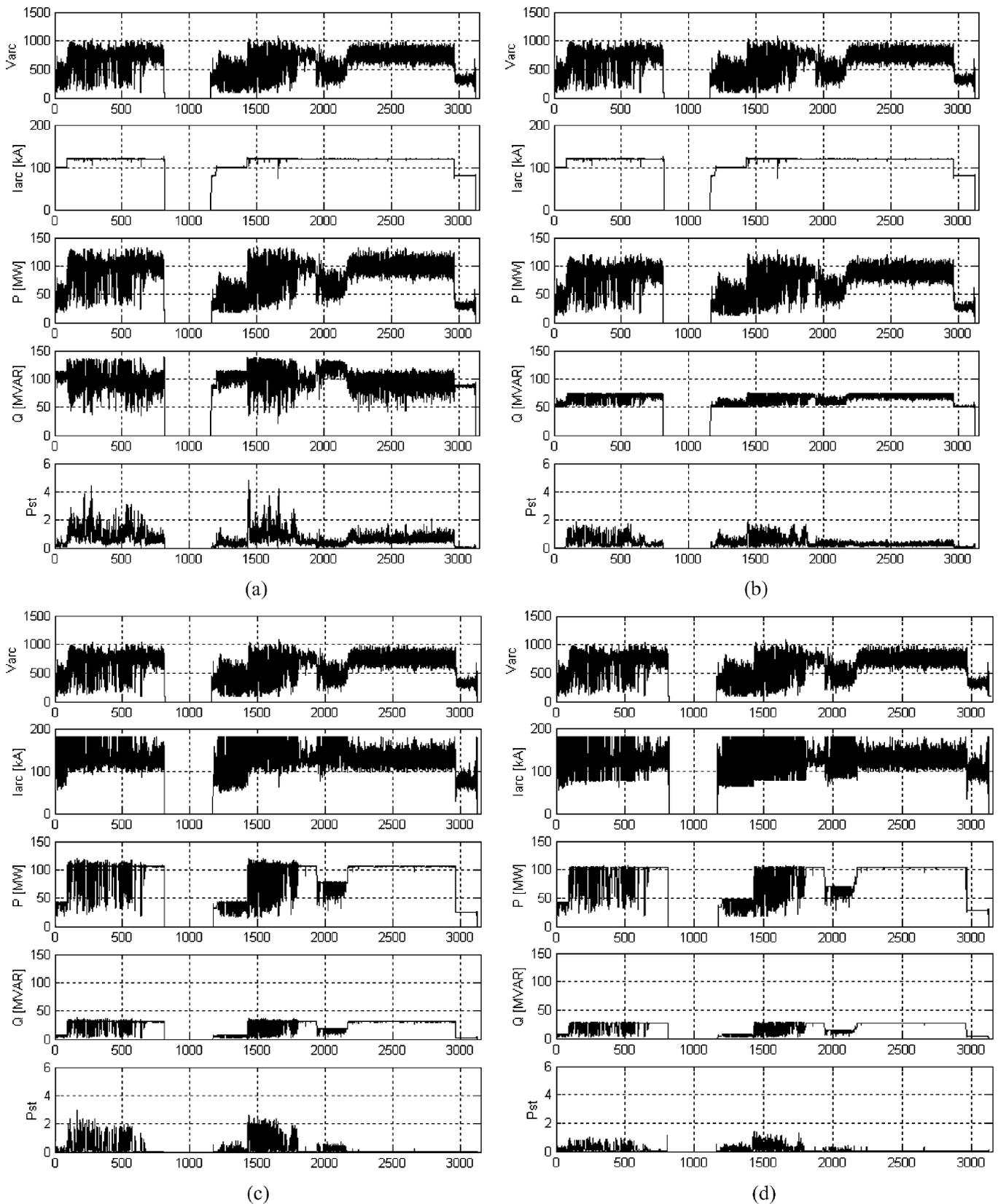
Fig. 10. (a) Simulation results for the classical supply with thyristor rectifiers. (b) Simulation results for the  $Q$  constant supply. (c) Simulation results for the chopper dc supply with constant power control. (d) Simulation results for the chopper dc supply with hysteresis on constant power control.
